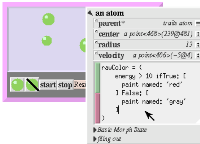
Figure 6. The user has selected one atom on which to experiment. The user changes the “rawColor” slot from a computed to a stored value by editing directly in the atom’s outliner.
