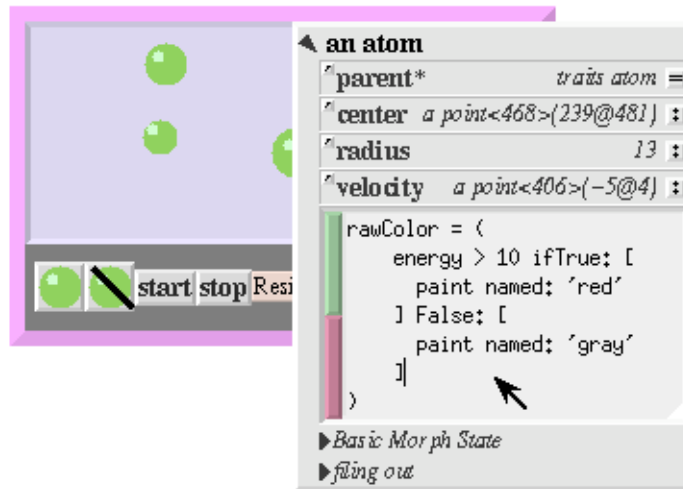
Figure 9. The user has selected one atom on which to experiment. The user changes the “rawColor” slot from a computed to a stored value by editing directly in the atom’s outliner.
